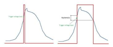
This mode can be used for both periodical and non-periodical input signals. Triggering voltage level can be set for rising, falling or both edges of input signal. Hysteresis can be set. One defined pulse or defined series of pulses can be generated after crossing of voltage level. One lasting pulse or lasting series of pulses can be generated during time when voltage is above/below voltage level.
